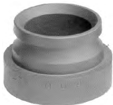
Figure No. 7320 2 1/2 male British Instantaneous 2 1/2 female threaded adapter Aluminum alloy
